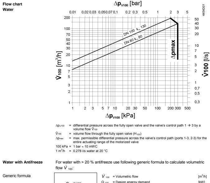
$\dot{V}_{100} = \frac{Q_{100} \cdot 3600}{c \cdot \Delta T \cdot \rho} [m^3 / h] \begin{pmatrix} \dot{V}_{100} &= Volumetric flow & [m^3/h] \\ Q_{100} &= Design energy demand & [kW] \\ \Delta T &= Temperature difference between flow and return & [K] \\ c &= specific heat capacity & [kJ/kgK] \\ \rho &= specific density & [kg/m^3] \end{pmatrix}$
