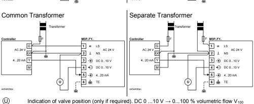
Indication of valve position (only if required). DC 0 ...10 V  $\rightarrow$  0...100 % volumetric flow V<sub>100</sub>
