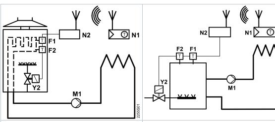
Wireless room temperature controller with receiver control of a gas-fired wall-hung boiler
