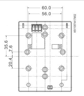
Room temperature receiver with mounting plate
